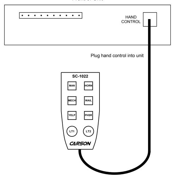
Note: Cable may be extended with ED1753 Hand Control Cable Extension Kit.
